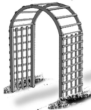
Put the posts back in the holes and check that the posts are plumb (straight up and down) with a level. If necessary, lift the posts back out of the holes and shovel in, or take out, gravel to correct any problems, and check again that the posts are plumb.
