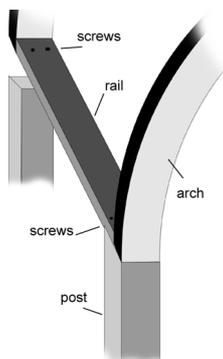
Drill two pilot holes through each arch rail into the top of each post and fix with two 75mm galvanised screws.
