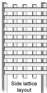
The vertical lattice (45mm x 20mm) can now be fixed to the horizontal lattice. This not only adds to the overall look, it also provides additional reinforcement.
