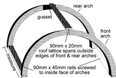
Unlike the rails, each roof lattice piece is screwed on top of the front and back arches, not between them, so take an overall measurement of the left rail and front and rear arch
