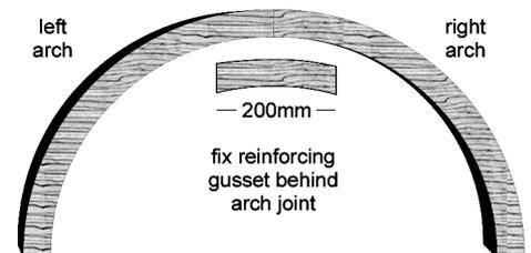
Follow the tracing with your jigsaw and cut out the gusset. Then cut out a second gusset, so there's one for both front and back arches.
