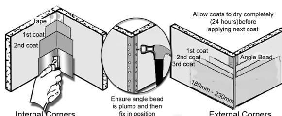
After attaching the metal corner strips use a 100mm broadknife to spread compound mix 75mm to 100mm out from the nose of the bead.
