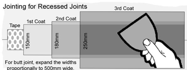
Do not apply the second coat until after the first has dried completely. First, hand sand off any excess and lumps from the first coat and then apply the second coat to a width of 180mm. Allow at least 24 hours to dry.
