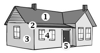
**Roof** - Paint all the ridge, hip and valley flashings by brush and then fill the large areas with a roller.
